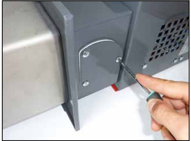
Disassemble seal cover located on the lower section of the burner
