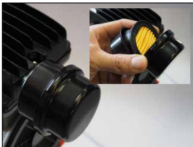
Cleaning compressor filter
