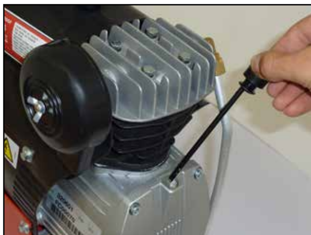
Checking oil levels in compressor
