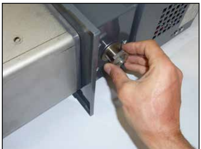
Set the pneumatic cleaning channel in the burner and gently secure using washer and low nut
