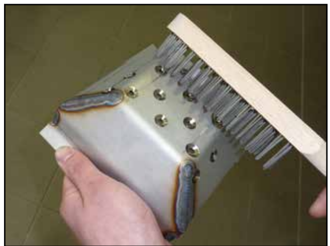
Example of cleaning the combustion chamber
