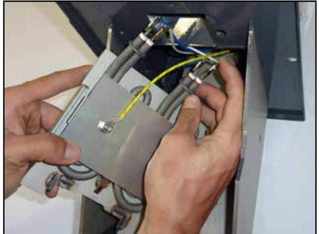
Mount connectors to every ignition coil (white and blue always together on one ignition body)
