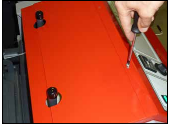
Return the back section of the machine hood to its place and fix securely
