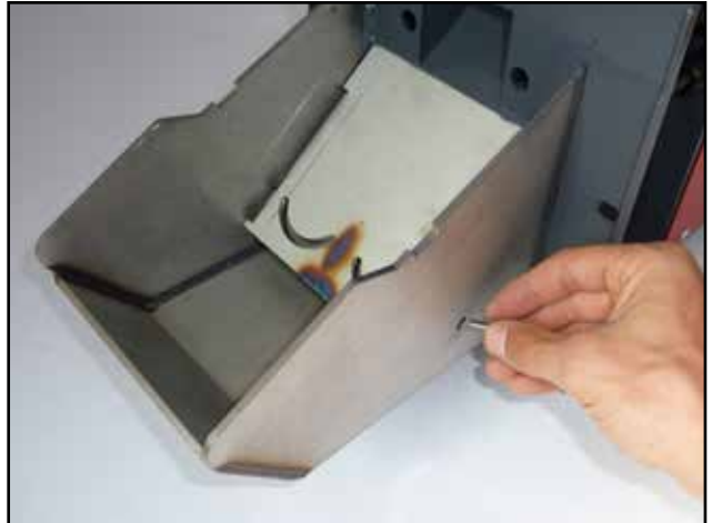
Screw out the M6 screws which hold the ignition coil board
