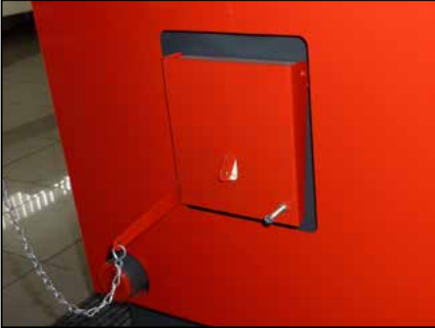
Closed flap for inflow of combustion air for DxxP, Pxx boiler
