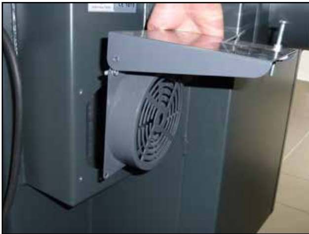
Disassembling flap for combustion air inflow
