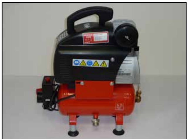
Amended compressor for pneumatic cleaning
