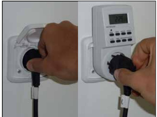
Connect the connecting cable to the wall socket, either directly or using a special timer with 8 A inductive load .... code: S0090 (Note – cannot normally be bought in shops)
