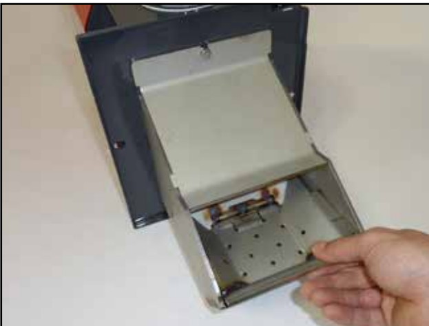
Insert new combustion chamber and check everything once again, tightening where needed
