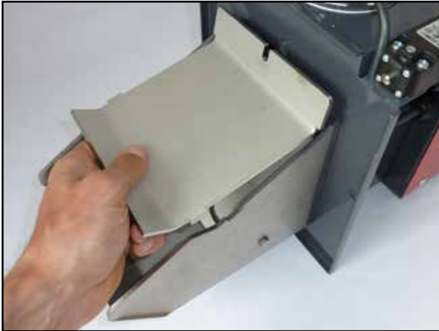
Loosen and screw out the M6 screw which holds the burner nozzle cover and remove the cover
