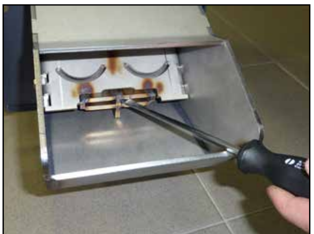
Example of cleaning the front part of the compressed air inflow channel
