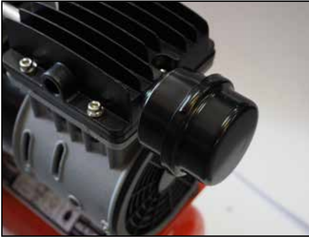
Photo of suction filter screwed onto compressor
