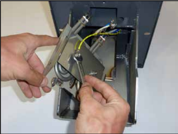
Insert the new board for holding the ignition coils into the burner while securely affixing the frame (green-yellow wire) under one of the nuts
