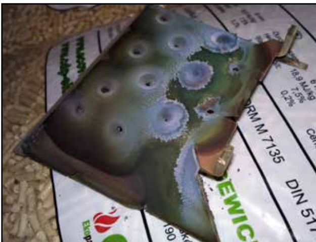
Slightly clogged apertures in combustion chamber after 4 months of use
