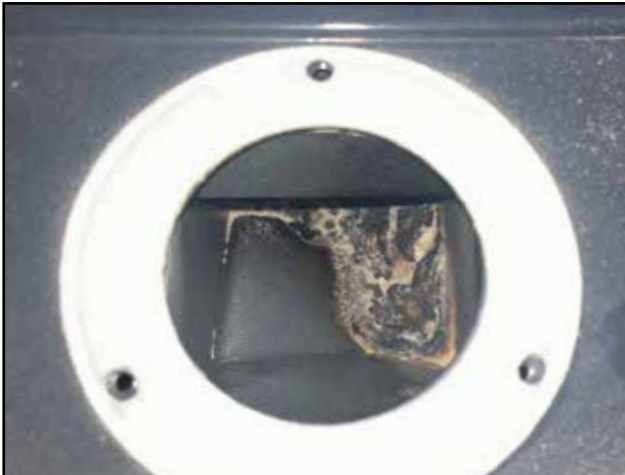
Clogging after 3 months use with crushed pellets with large amount of dust
