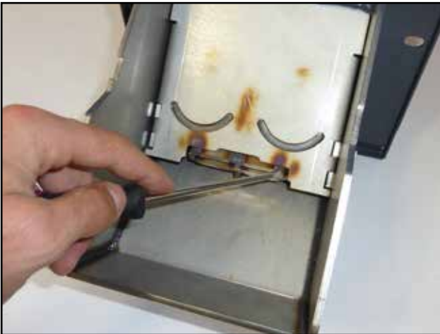
Insert ignition coil board in its place and centre the pneumatic cleaning channel in its designated place
