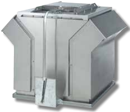
Smoke extract fan RDM 56: 400°C / 120min. RDM 57: 600°C / 120min.
